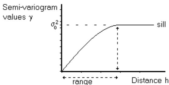
Figure 11.4: Example of a spherical semi-variogram model.  $\sigma_0^2$  is the total variance of input data.  $\gamma$  are semi-variogram values.
