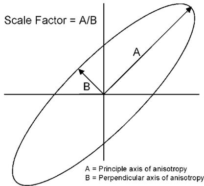
**Figure 11.6:** Explanation of the scale factor and the principle axis and perpendicular axis of anisotropy.
