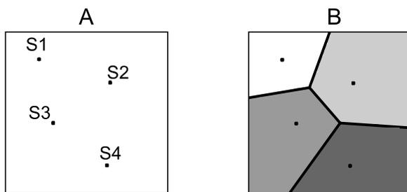
**Figure 11.3:** (A) An input point map. (B) The output map obtained as the result of the interpolation operation applying the Nearest Point interpolation method.
