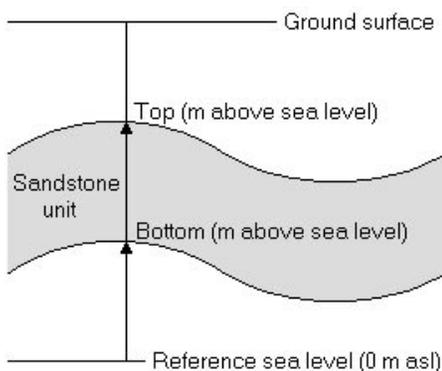
**Figure 11.1:** Schematic representation of a potential oil reservoir. Given are the vertical distances towards the top and the bottom of sandstone unit.
