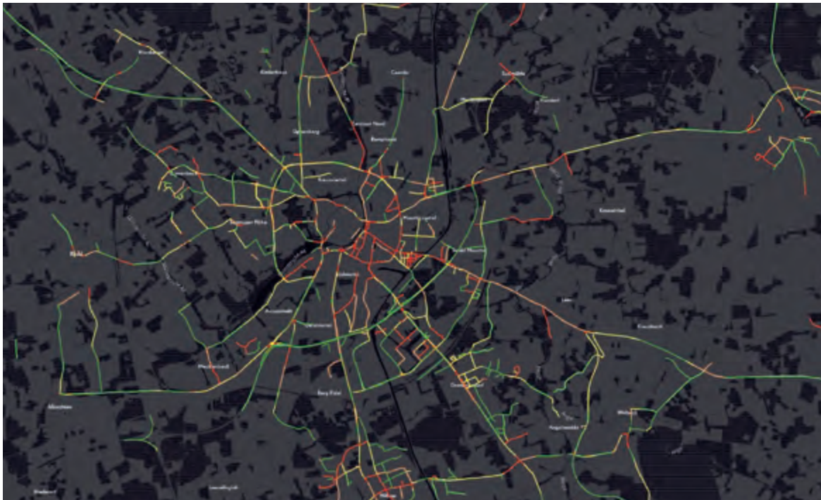
Comparison between speed limits and average velocities (Red: < 50% of limit, Green: > 80% of limit)
